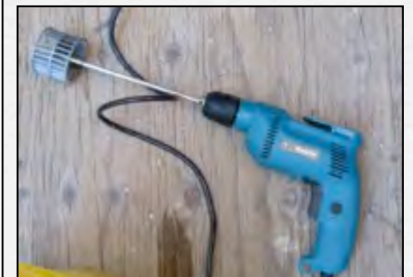
Hurricane/rotary mixer attached to drill
