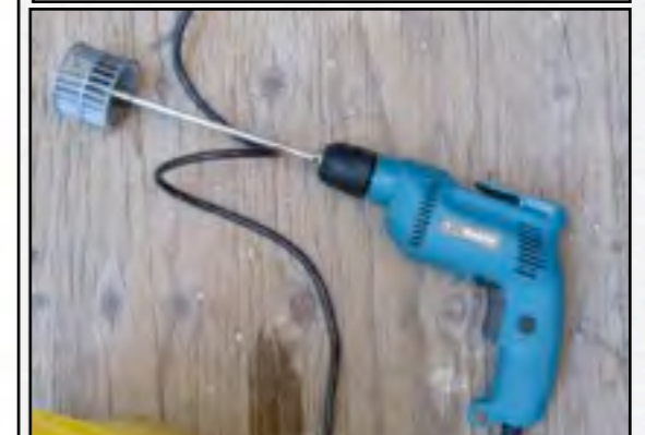
Hurricane/rotary mixer attached to drill
