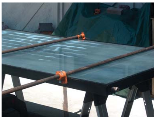
The first Nansulate® coated solar panel. The interior case is coated with nine coats of Nansulate® Solar
