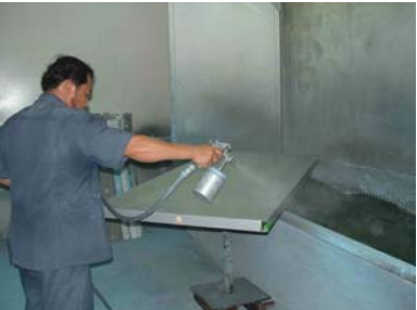
Technician applies Nansulate® Translucent PT to aluminum panels
